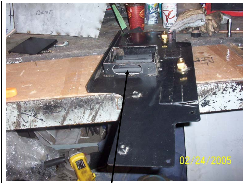
Front panel. Cut hole as shown to add hose adaptor to front foot panel.
