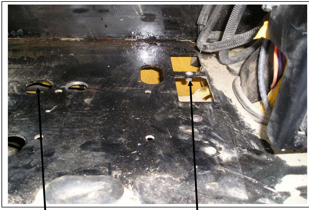
Drain tube will align over this hole.
