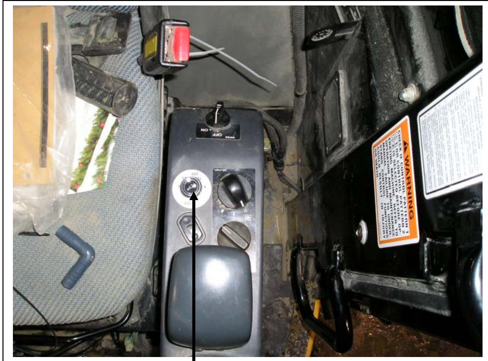
Thermostat installed on control arm beside operator.
